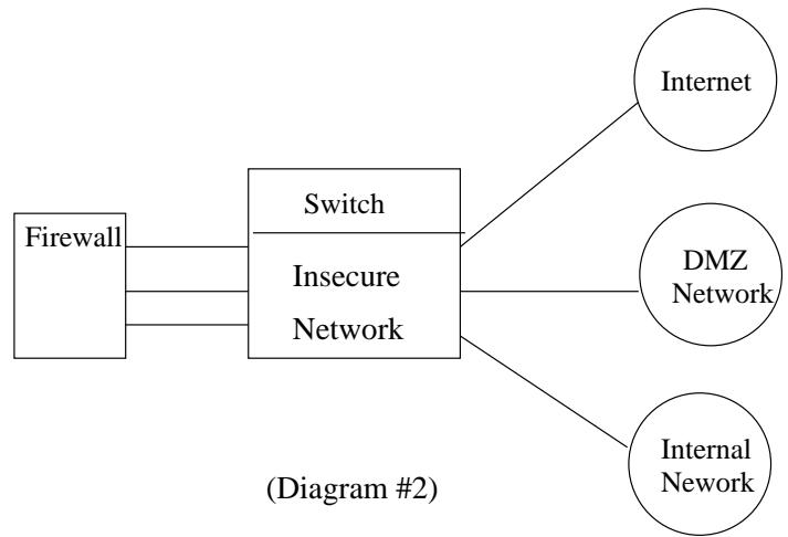
As you can see in diagram #2, a compromise of the switch resulting in a reconfiguration of its VLANs may severely reduce, or even mitigate the effectiveness of the firewall. Other forms of attack may attempt to take out the
